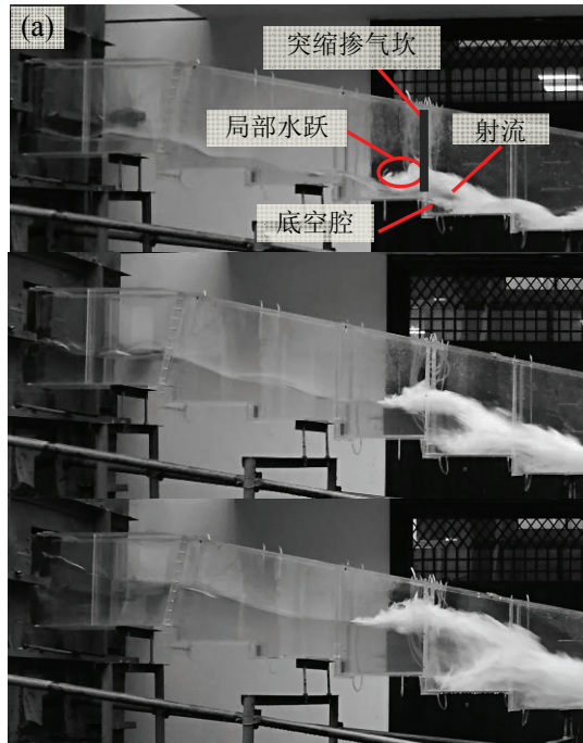
图3 突缩掺气坎流态 ( b/B = 0.667, q = 0.09, 0.24, 0.56\text{m}^2/\text{s} )
